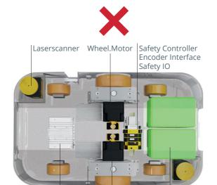
Controll Unit | Servo Drive | Safety encoder | Batteries
