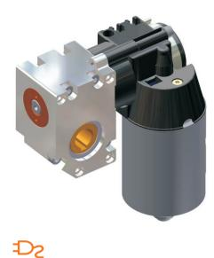
Powerful 24 V DC motor with two worm gears and a planetary gear. High reduction ratio makes precise control and position setting possible.
